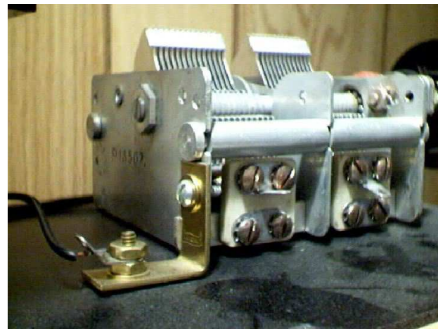
This is my common to the frame or body of the capacitor.
