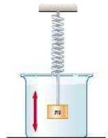
Fig. 3. A mechanical analogous to the RLC circuit – a block-spring system moving in a viscous medium.
