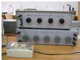
Fig. 7. The decade coil, the decade resistor and the capacitor with its charging system.
