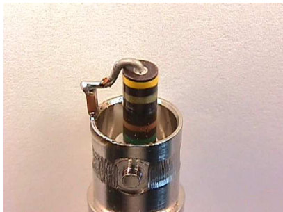
Figure 1. Test Circuit for Measurement of Capacitor Self-inductance and ESR
