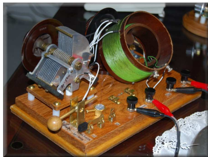
View from behind with my cat's whisker crystal detector, SPDT knife and 1N34A diode.
